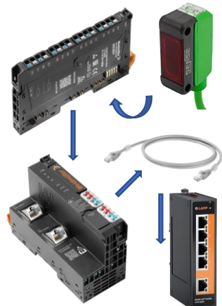
Sensor + Módulo ED + CLP + Patch Cord + Switch industrial
