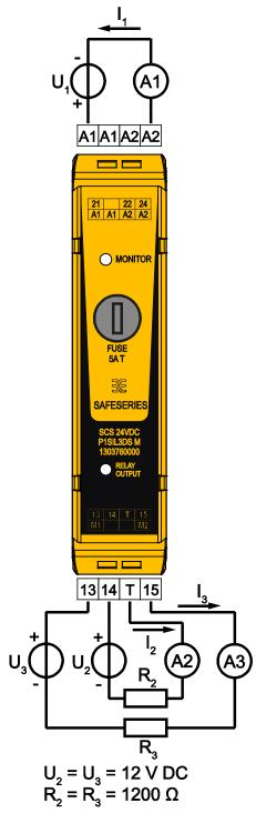
(The illustration shows the front view of the parts (order number) 1303760000 SCS 24VDC P1SIL3DS M and the 1304040000 SCS 24VDC P1SIL3DS MG3. The monitoring circuit is not applicable for the part 1303890000 SCS 24VDC P1SIL3DS).
